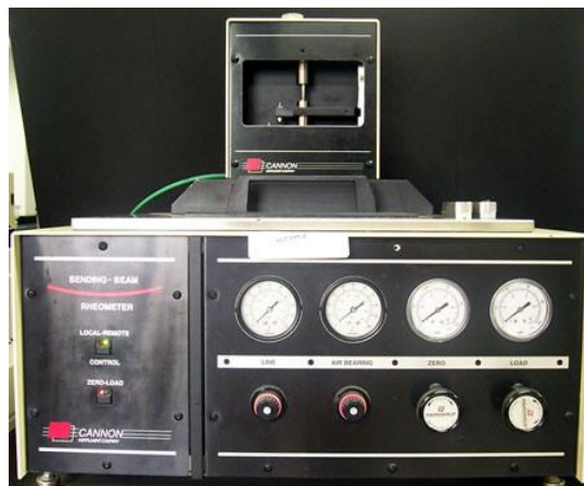
Figure 3-5. Bending Beam Rheometer.
