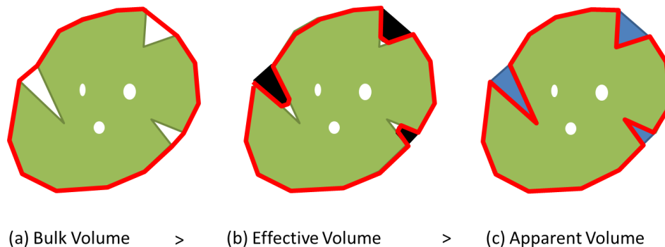
Figure 3-10. Schematic of the Definitions of Volume (within Red Outline) for Aggregate Specific Gravity.
