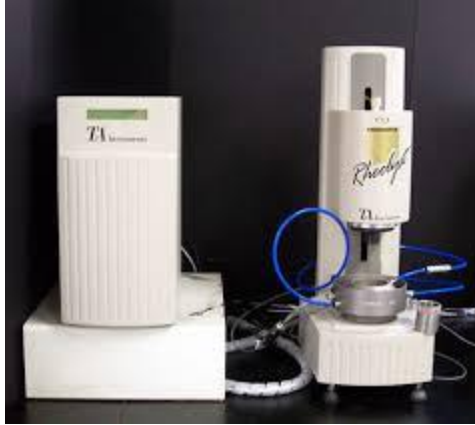
Figure 3-4. Dynamic Shear Rheometer.
