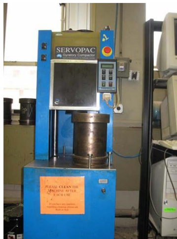
Figure 3-13. Superpave Gyratory Compactor.
