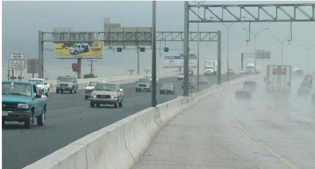
Figure 1-3. PFC (Left Side) Reduces Splash and Spray in Wet Weather.
