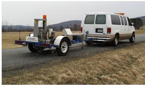
Figure 4-5. Falling Weight Deflectometer.
