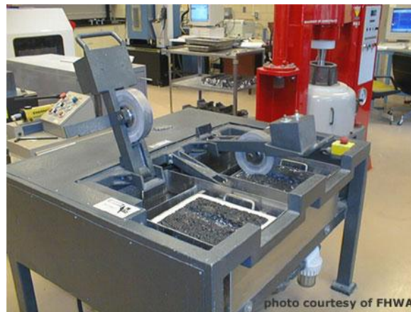
Figure 3-16. Hamburg Wheel Tracking Test.
