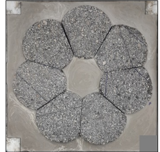
In between Wheel Path Cores
