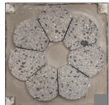
In between Wheel Path Cores
