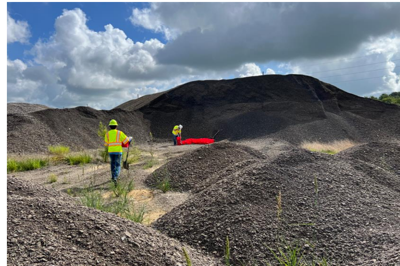
Waco RAP, Big Creek Materials Milled from PFC surface Non-fractionated Sampled on June 26 th , 2024
