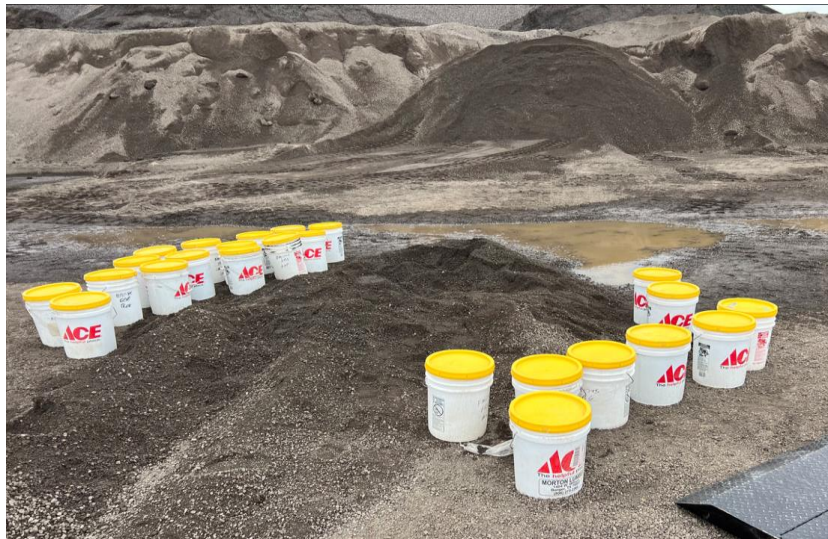
Fort Worth (FW) RAP, Texas Materials Milled from IH35 Fractionated Sampled on Feb. 8 th , 2024
