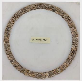
Aggregate polished using Micro-Deval, TxDOT test procedure.
